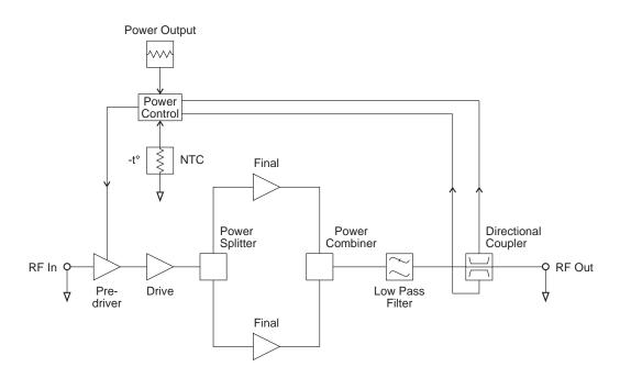
Figure 2.1 T838 High Level Block Diagram
