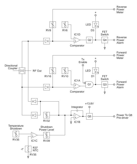
Figure 2.3 T838 Control Circuitry Block Diagram
