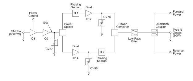
Figure 2.2 T838 RF Circuitry Block Diagram
